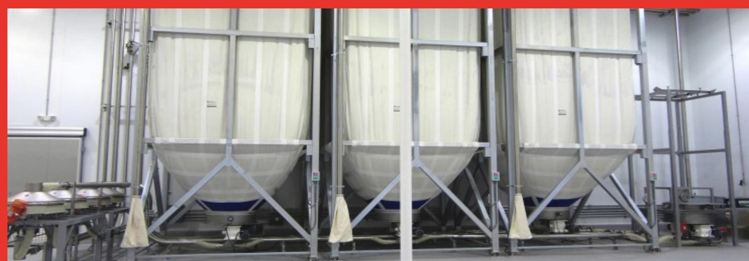
Fabric silos are robust, modular galvanized or painted steel constructions designed to meet specific client needs.
