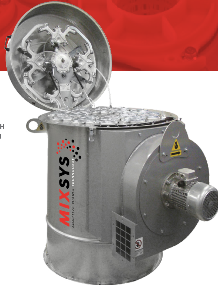
Quick-change cartridge filter replacement system
