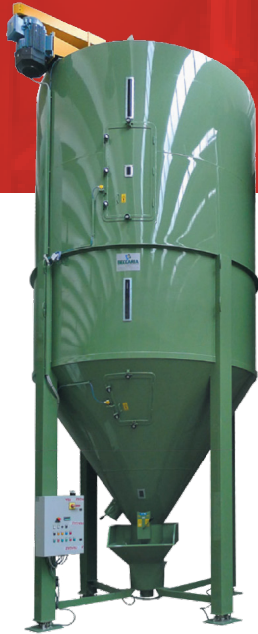
Mixing silo 45 m 3 on load cells
